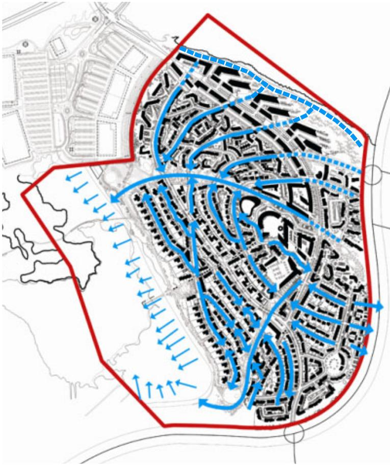
Urriðaholt sustainable drainage system - green wedges provide retention for severe storm events
