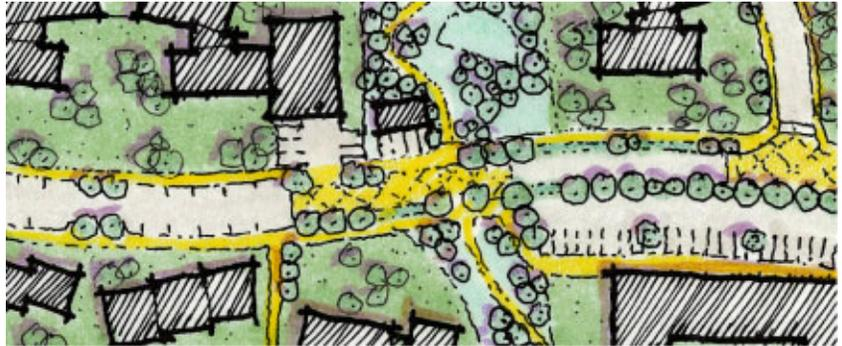
Each residential street is given a unique character, a variety of traffic calming methods are used to reinforce this variety. The Diagonal Connector meanders slightly to continually change the vista for pedestrians and drivers, tabletops slow traffic at pedestrian crossings and intersections
